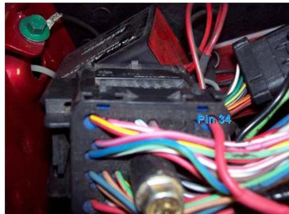
17) Remove the tape securing the WOT box connector. Plug in the WOT box, and mount securely.
