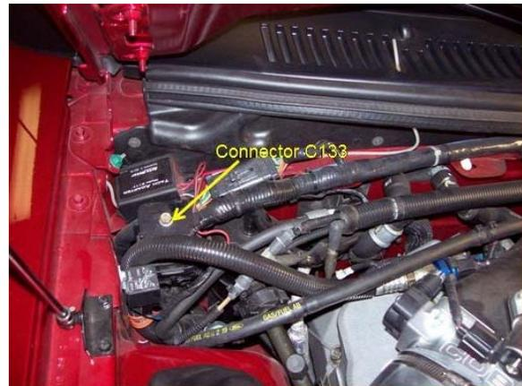
15) Making sure to leave enough room to connect on both sides, cut the red wire.
