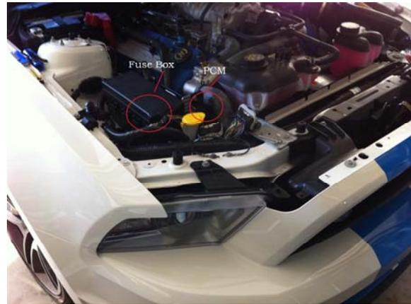
8) The PCM is located in the front of the engine compartment on the passenger side. Unplug all 3 cam-lock connectors from the PCM by unlocking the grey levers and pulling the connectors out.
