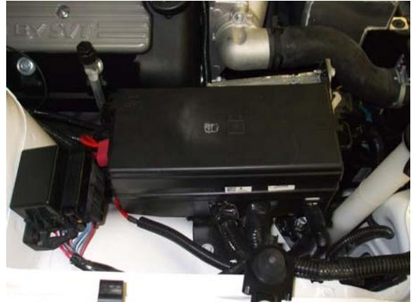
14) Remove the 4 bolts in the center of the BEC and remove the top of it to allow access to the connectors underneath.
