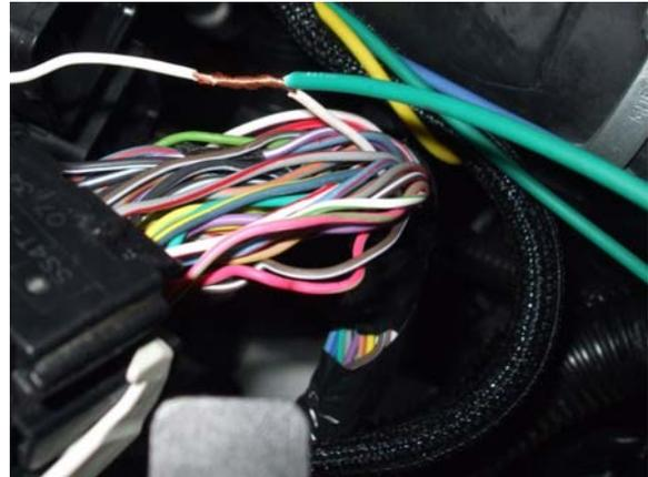
11) If you haven't already, remove enough of the loom behind the middle connector to access the wires. Splice the **BLUE WOT Box Wire** into the **WHITE** wire on pin 17 of the **MIDDLE CONNECTOR**. Use the N2MB recommended soldering technique. Re-install the loom on all connectors accessed and tape securely with electrical tape.
