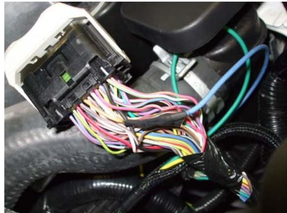
12) Remove enough of the loom behind the bottom connector to access the wires. Splice the **YELLOW WOT Box Wire** into the **BLACK/PINK** wire on pin 47 of the **BOTTOM CONNECTOR**. Use the N2MB recommended soldering technique. Re-install the loom and tape securely with electrical tape.
